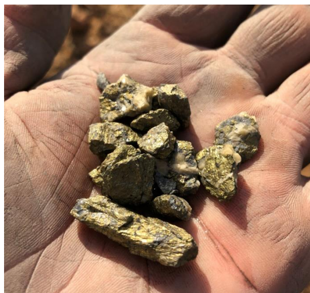
Figure 3. Chalcopyrite mineralisation from RC drill chips of drillhole WRCR021.
