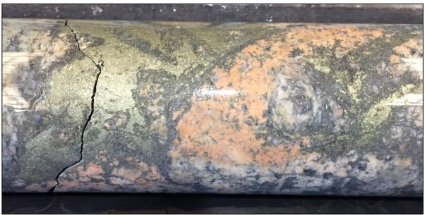
**Figure 4.** Breccia-hosted copper mineralisation west of the Corvette deposit, comprising 5.8 metres at 1.97% Cu & 179ppm Mo, photographed from ~170 metres down hole in 23MYDD434 (ASX MAG 6 December 2023).
