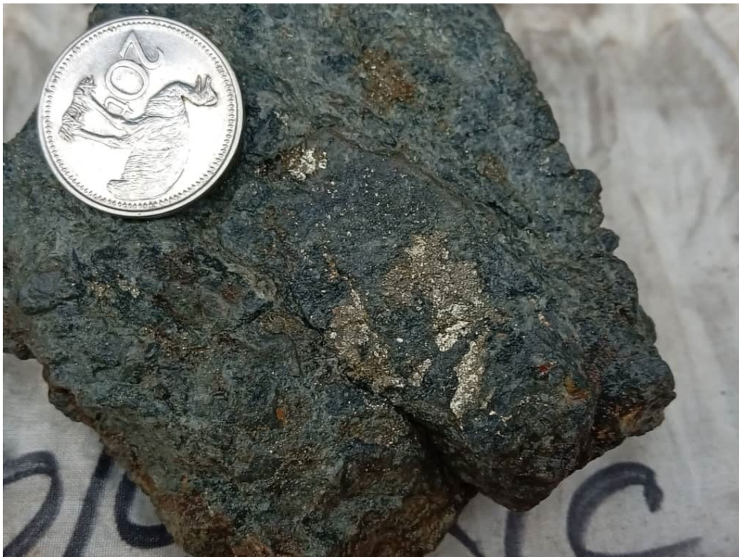
Figure 1: Outcrop Sample 702110 (0.11% Cu, 0.04 g/t Au, 4.3 ppm Mo) – Visible sulphides in a sheared breccia of andesitic volcanic sediment from North Agadul access corridor.
