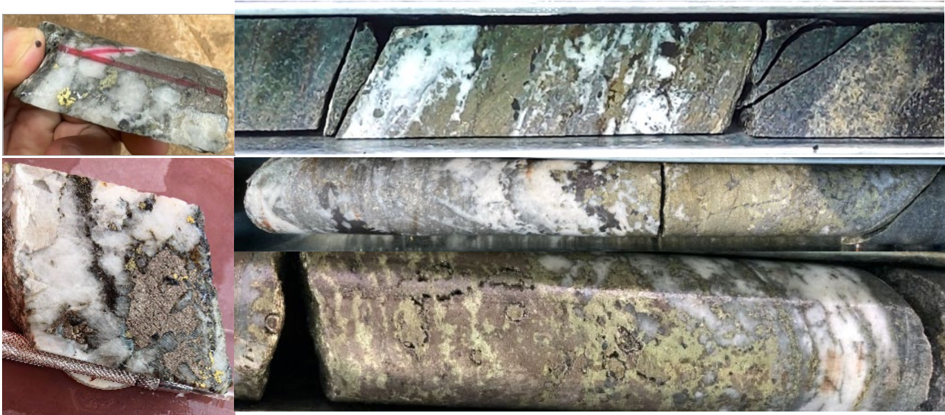
Figure 6 | Mineralised veins in Memot diamond core. Quartz veining with Pyrite, Arsenopyrite, Pyrrhotite, Chalcopyrite and Sphalerite sulphides. Left Hand Side photos: DD24MMT243 - 1m @ 2,090.00g/t Au from 130m. Right Hand Side top to bottom DD21MMT001 - 1m @ 8.91g/t Au, 2.16% Cu from 48m, DD22MMT013 - 0.4m @ 17.70g/t Au, 230g/t Ag, 2.78% Cu, 0.56% Pb and 1.74% Zn from 190m and DD21MMT006 - 1m @ 25.4g/t Au, 73g/t Ag, 1.81% Cu, 0.1% Zn
