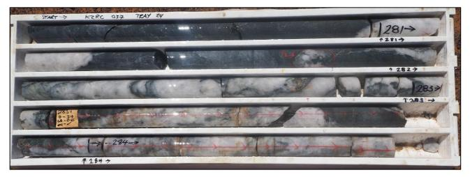
Figure 4. Part of sulphide mineralized quartz vein, hole 17KZRC037
