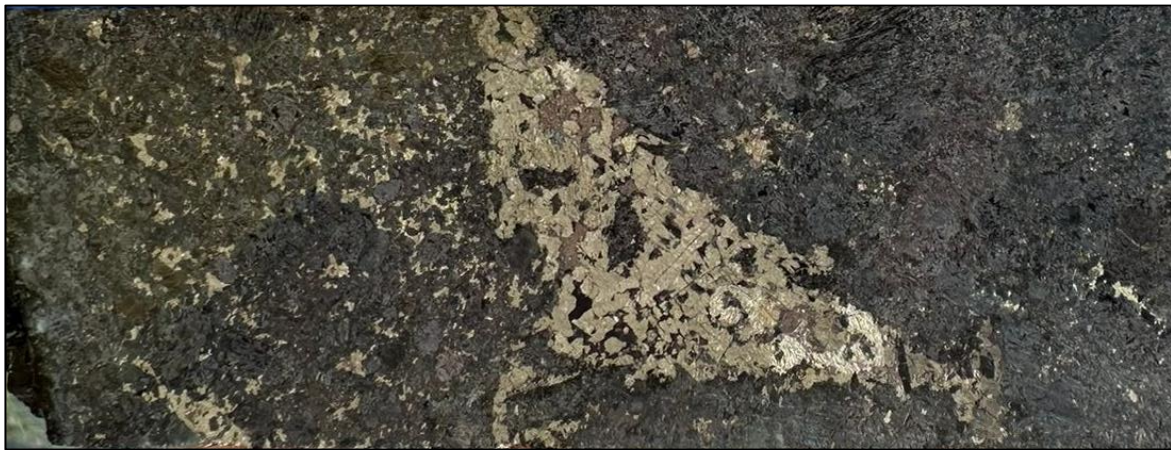
Figure 6. Blebby and disseminated magmatic sulfide rich in coarse-grained pyrrhotite, pentlandite and minor chalcopyrite from SWD009 (from 52 m), PQ core diameter 85mm (8.5cm).
