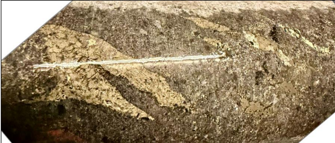
Figure 5. Immiscible sulfide blebs within the gabbro host rock. Rich in pyrrhotite with moderate pentlandite and minor chalcopyrite from SWD009 (from 52.2 m), PQ core diameter 85mm (8.5cm).
