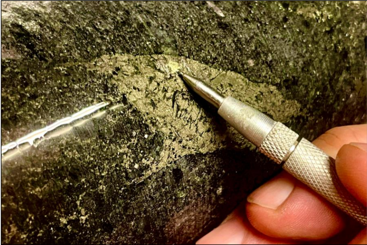
Figure 3. Blebby and disseminated magmatic sulfide from SWDD009 (from 52.2 m), PQ core diameter 85 mm (8.5 cm). A sulfide bleb shows chalcopyrite (yellow) associated with pentlandite (highly reflective brassy yellow) within a dominant pyrrhotite matrix. The bleb is surrounded by a thin reaction rim of dark minerals (likely magnetite), interpreted as a reaction feature formed where the immiscible sulfide liquid interacted with the surrounding silicate–oxide melt.
