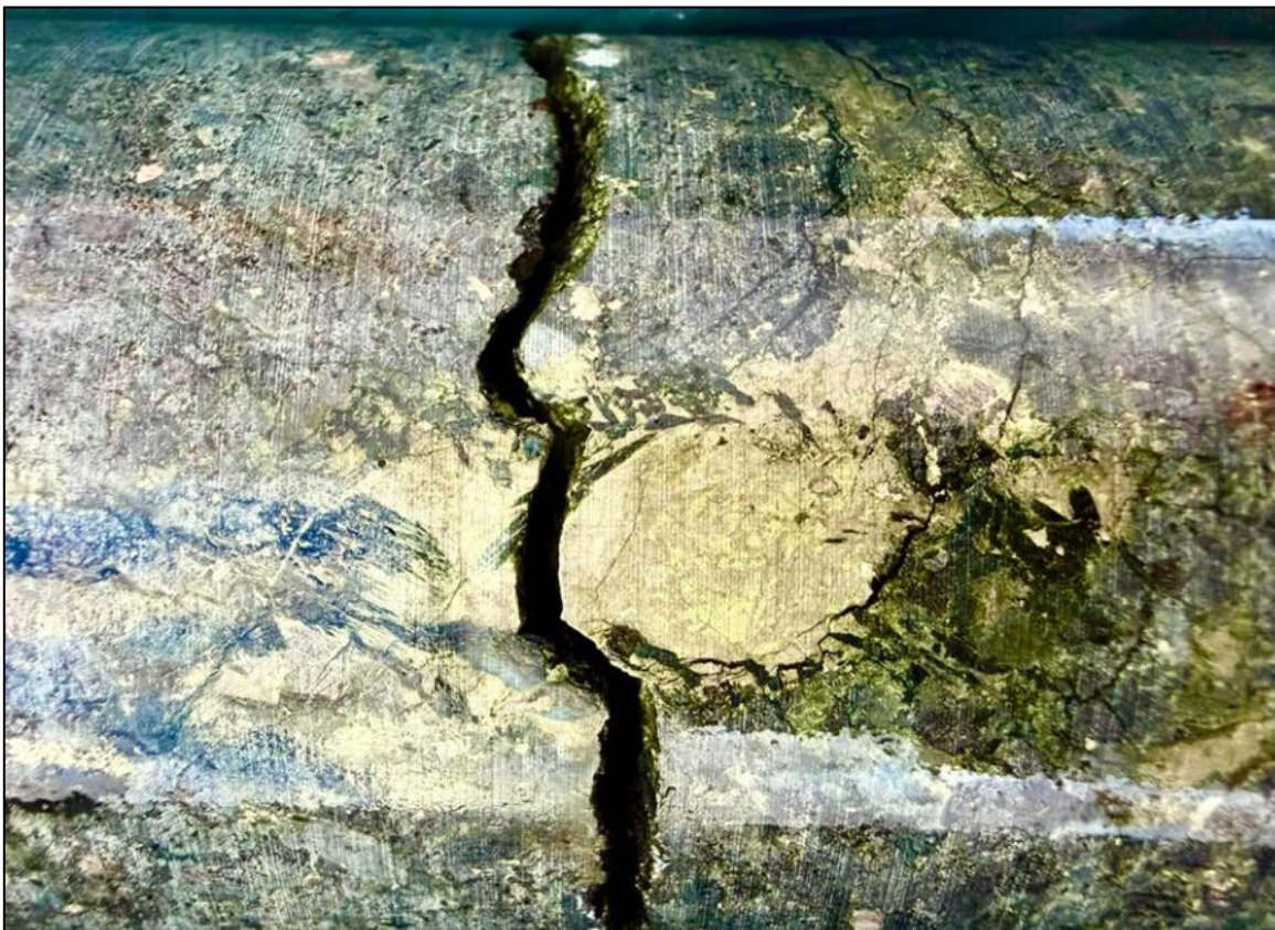
Figure 4. Blebby magmatic sulfide rich in chalcopyrite (yellow), pyrrhotite (brassy brown) and pentlandite (brassy yellow) from SWD009 (from 65.2 m), PQ core diameter 85mm (8.5cm).
