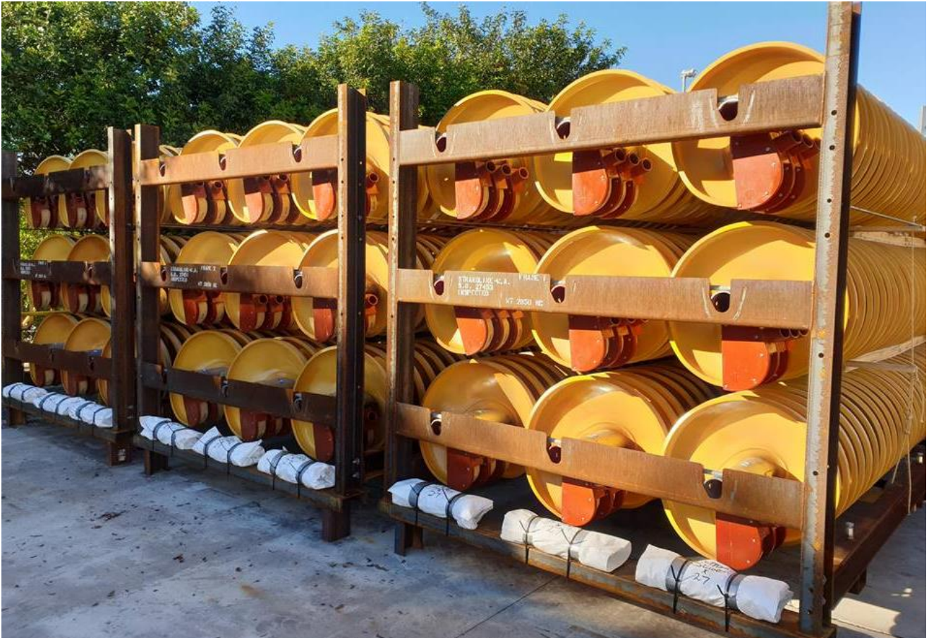
Figure 1 Coburn Project Manufacturing of Long-lead Spirals Equipment for the Processing Facilities (ahead of schedule)
