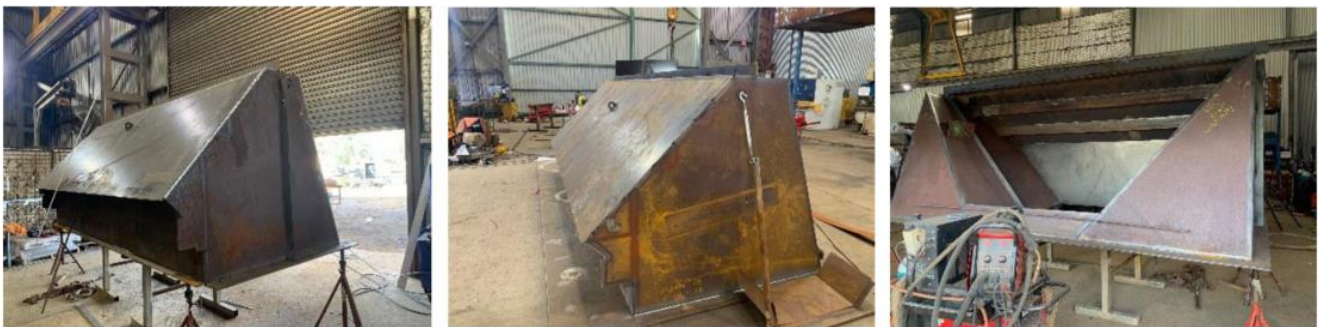
Figure 8 Coburn Project Fabrication of Dozer Mining Units progressing in WA
