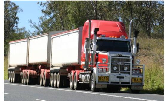
Image: Typical Triple Road Train Configuration
