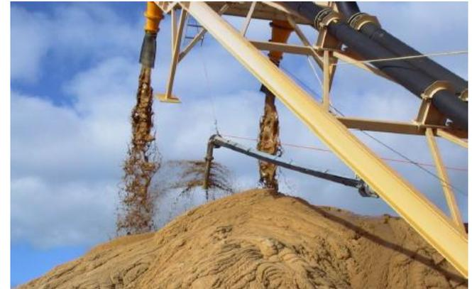
Image: Typical Co-disposal of Sand Tails and Slimes
