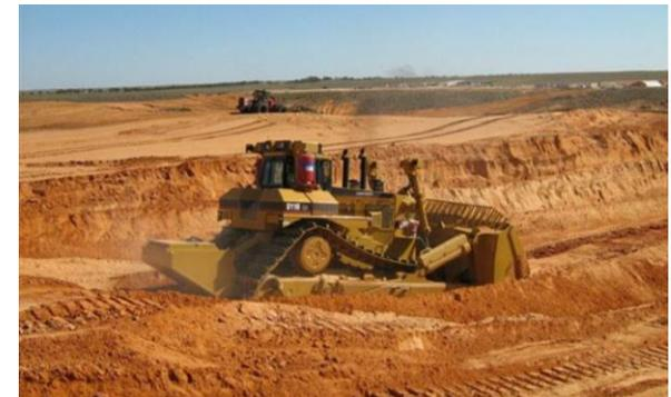
Image: Conventional Dozer Push Mining Method
