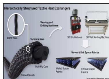
Fig. 3 Hierarchically structured textile heat exchangers — CNTF yarn to woven & knit spacer fabrics.
