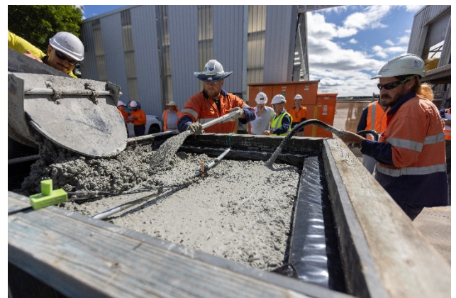
Figure 5: AusPozz™ concrete hotbox demonstration pour and temperature monitoring
