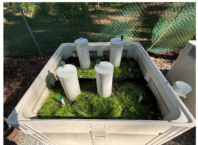
Figure 9: Simulated landfill configurations at Griffith University
