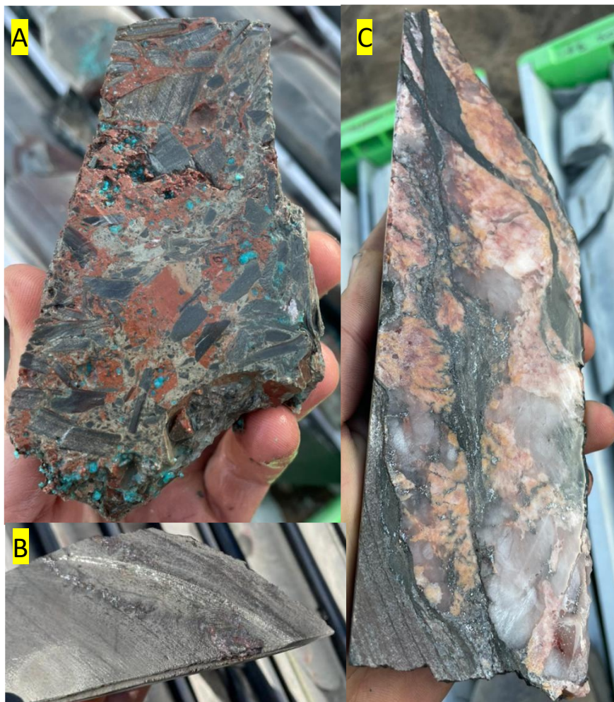
Figure 1. Examples of mineralisation intersected in NCP10. (A) hydrothermal breccia with chrysocolla (and fine-grained chalcocite) mineralisation, (B) chalcocite mineralisation on fracture planes, (C) chalcocite mineralisation (silver metallic colour) in complex quartz veins.
