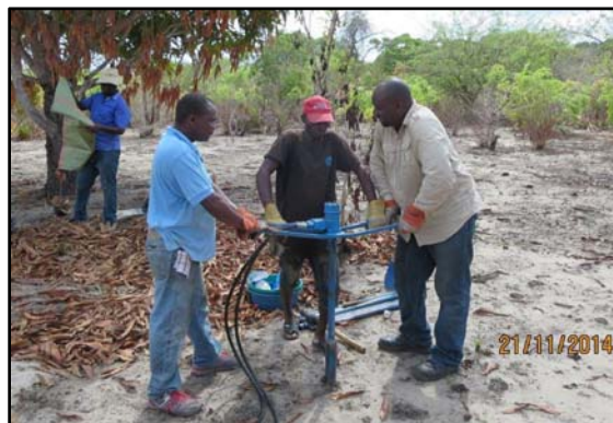
Figure 6. Auger drilling at the Madimba Prospect.
