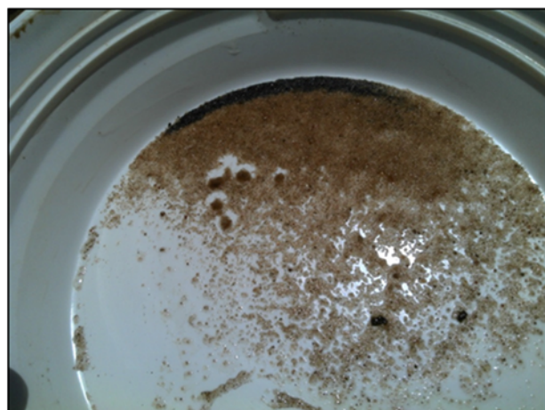
Figure 4. Pan sample from outcrop at roadside cutting estimated to contain 2 to 4% THM. Heavy mineral is located on the top of the pan as the dark coloured or black grains.
