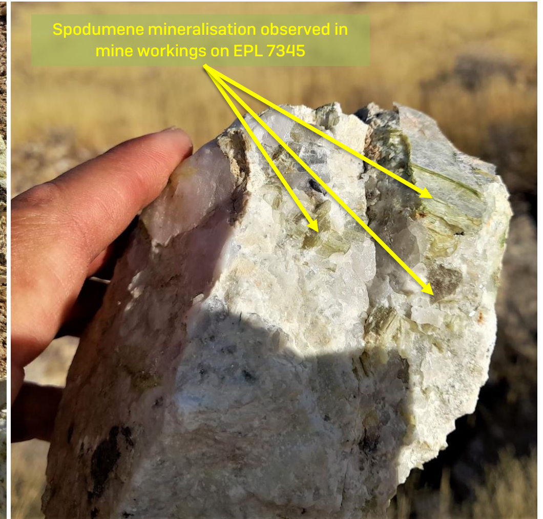
Figures 1 and 2: Samples containing altered spodumene, coloured in pale green, collected during the October 2022 due diligence field sampling campaign at the Uis Project
