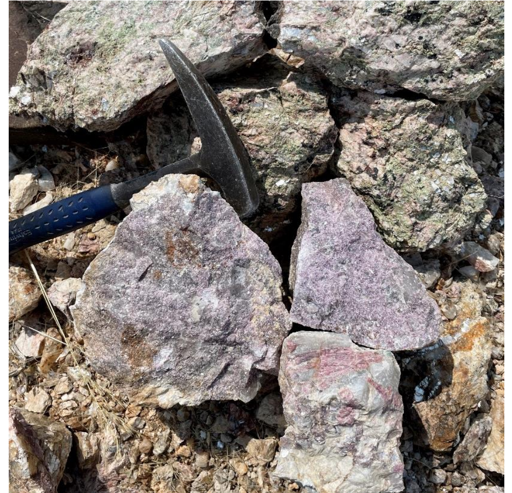
Figure 4: Photograph of rocks containing visible spodumene and lepidolite mineralisation collected from the Uis Project
