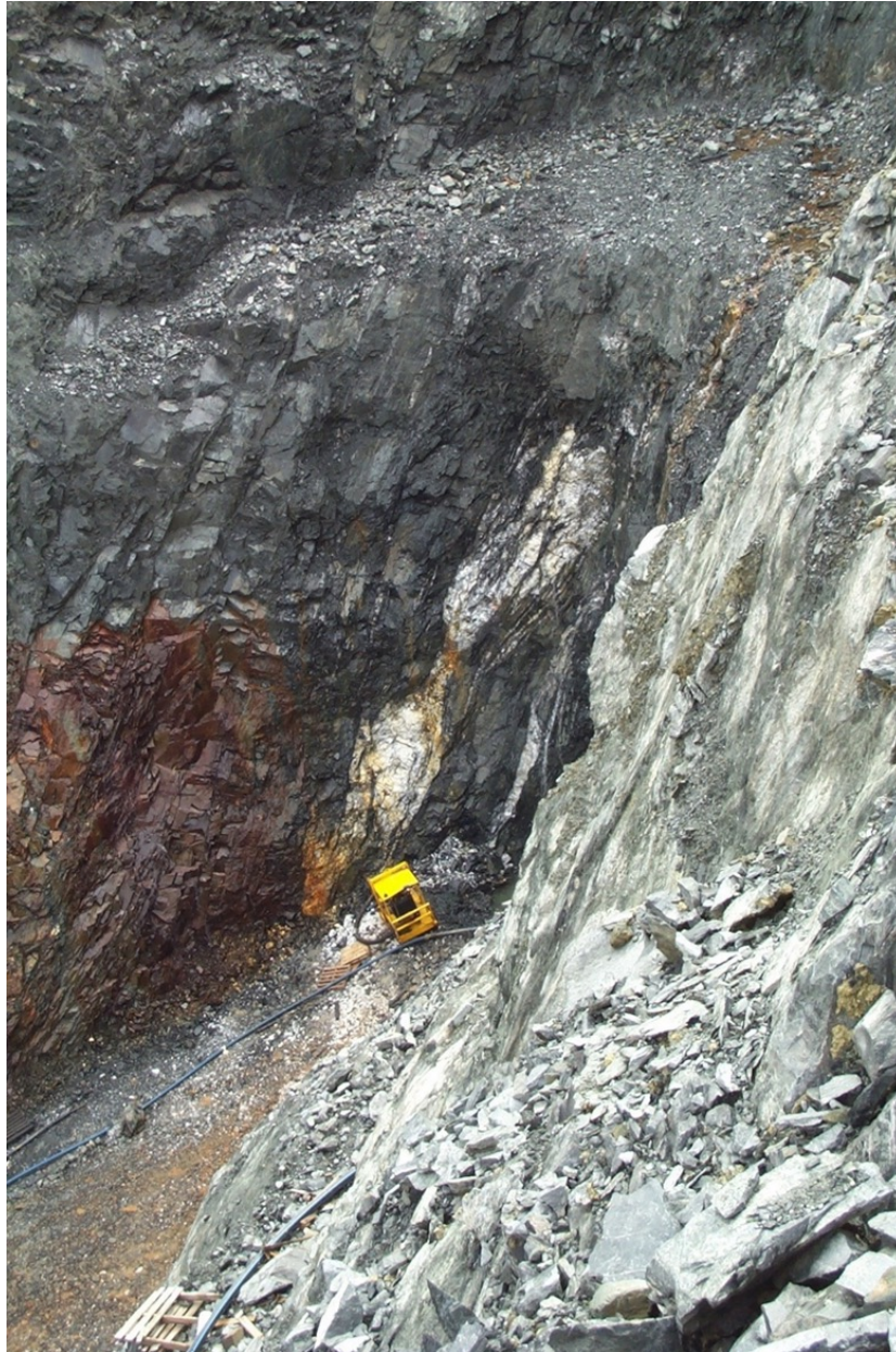
Figure: High grade ore zone in the Daisy Open Pit showing the pinch and swell of the veining.
