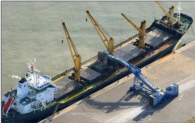
Figure 10: Example Mobile Ship loader Unit
