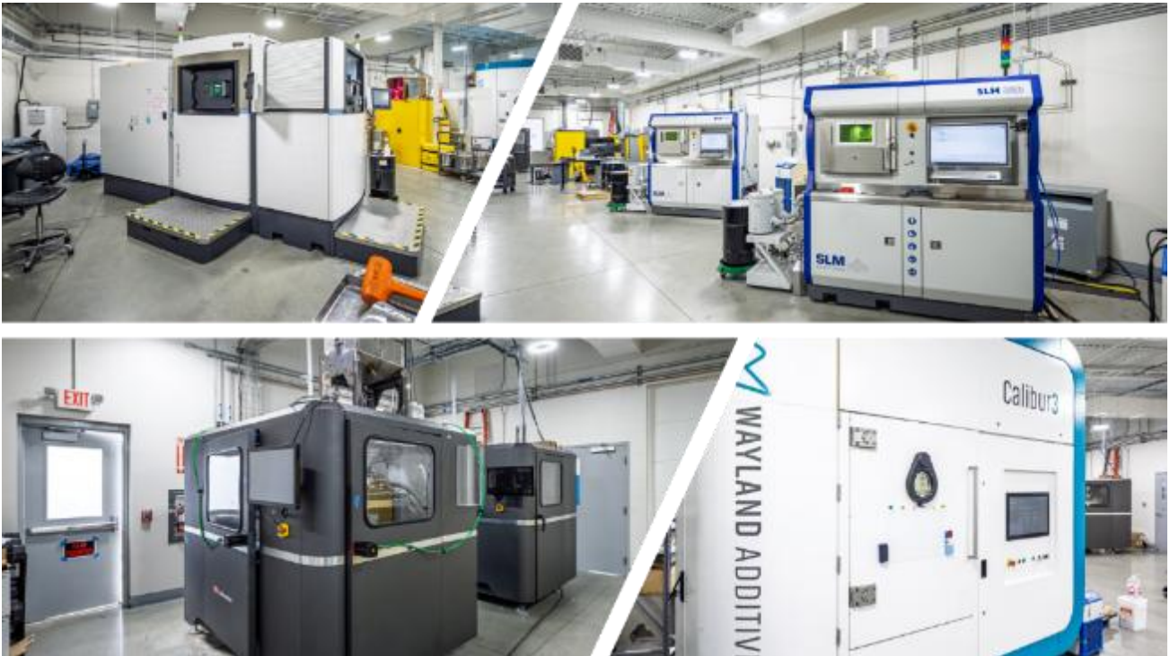
Figure 9, clockwise from top left: 1x EOS LPBF machine, 2x SLM LPBF machines, 1x Wayland Additive eBeam machine, 2x Desktop Metal binder jet machines
