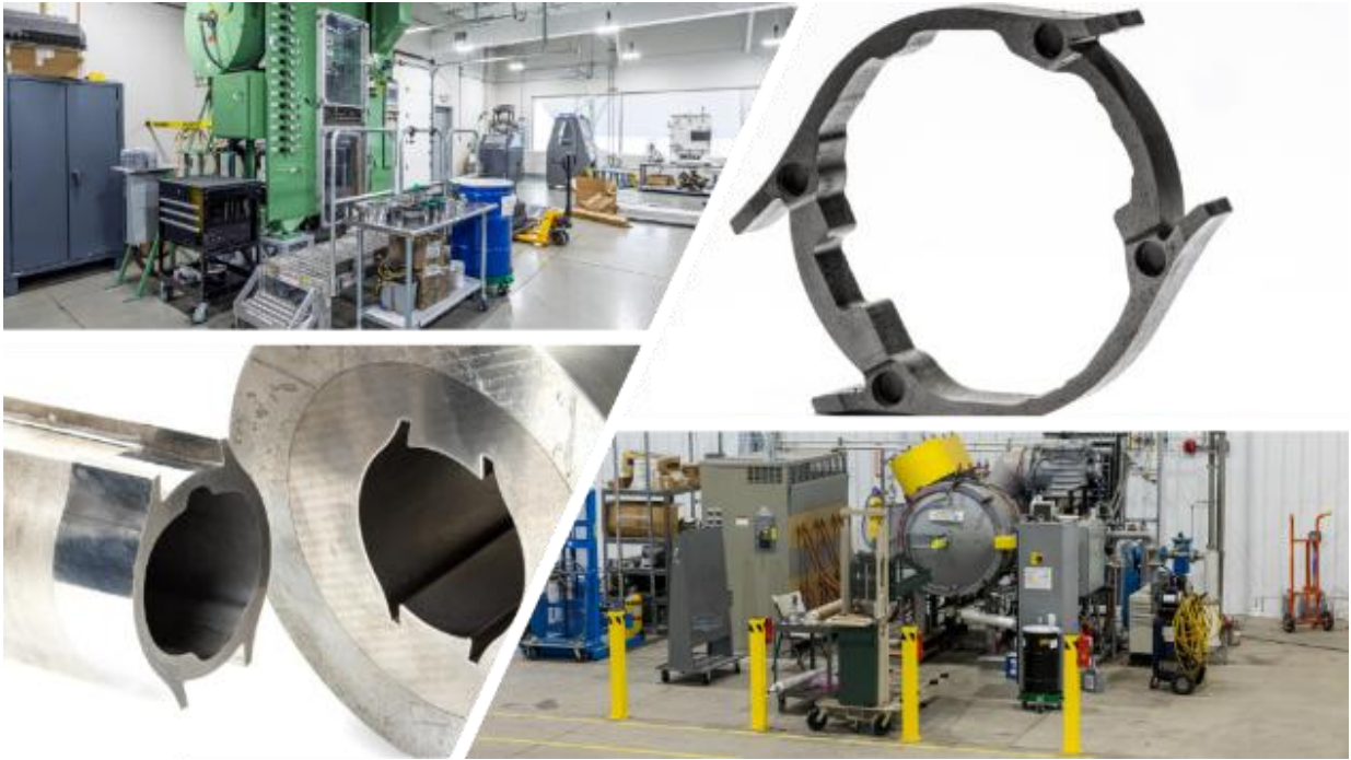
Figure 7: Anticlockwise from top left – uniaxial press, press die set, sintering furnace, finished component
