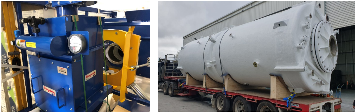
Figure 1 Equipment for vanadium electrolyte production – L-R bag unit and electrolyte tank
