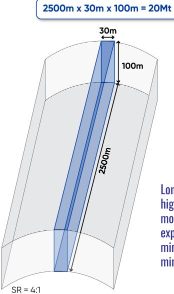
Long and steep higher waste movement and expect a higher mining cost. Deeper mining.
