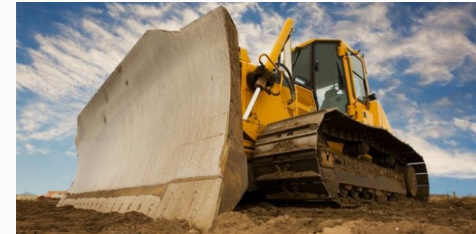
Image: Conventional dry mining using dozer push method
