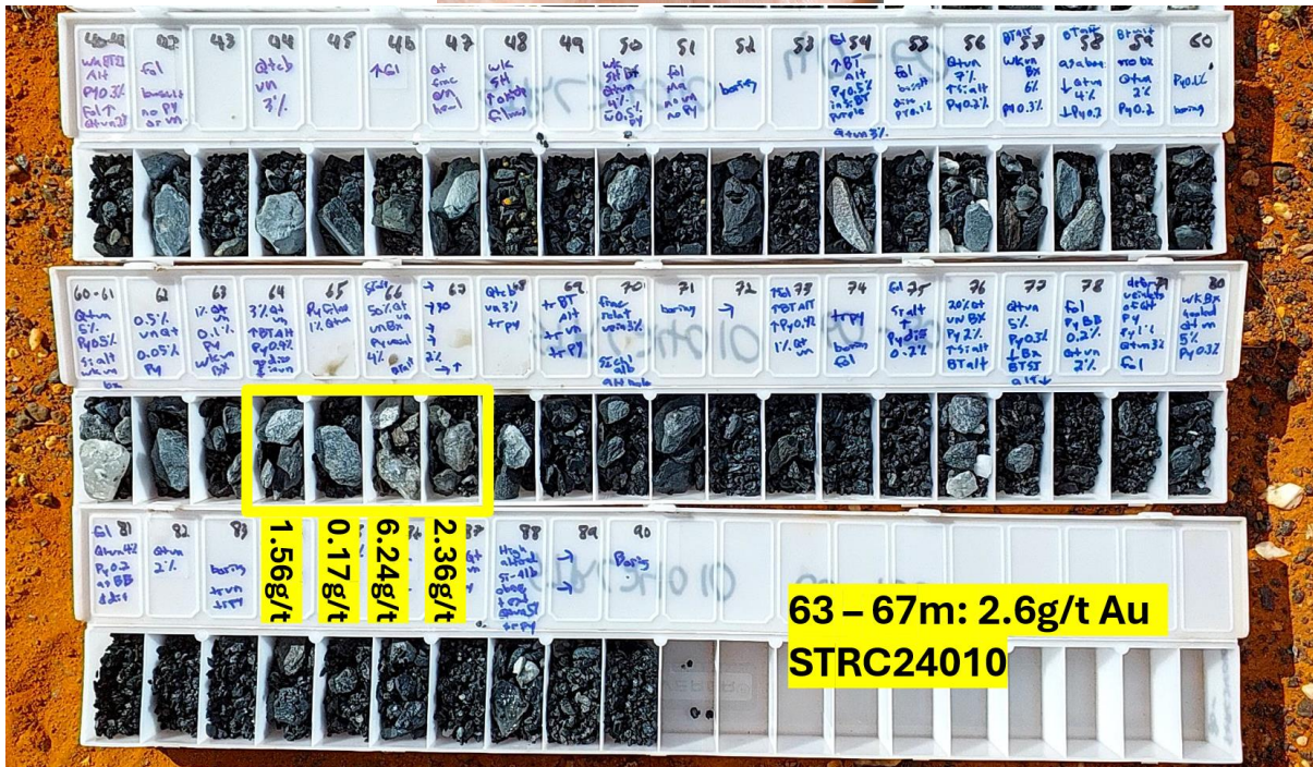
Figure 6 – Above: RC chips in hand from 65-66m from Stirling STRC24010 returning 6.24 g/t. Below: Chip tray showing significant intercept at Stirling in STRC24010 (4m at 2.6 g/t Au from 63m).
