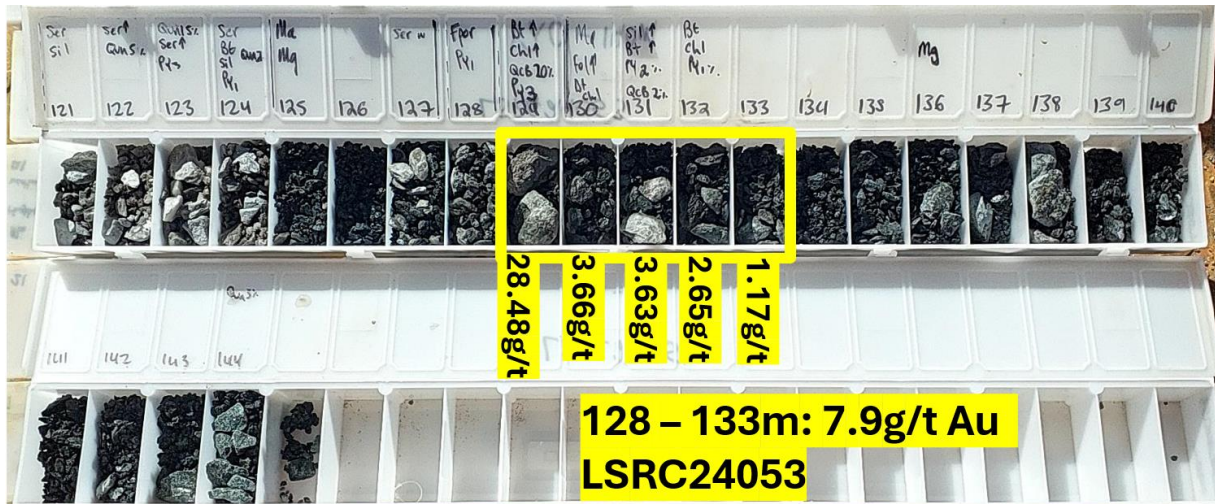
Figure 7 – Chip tray showing significant intercept at Pericles in LSRC24053 (5m at 7.9 g/t Au from 128m).
