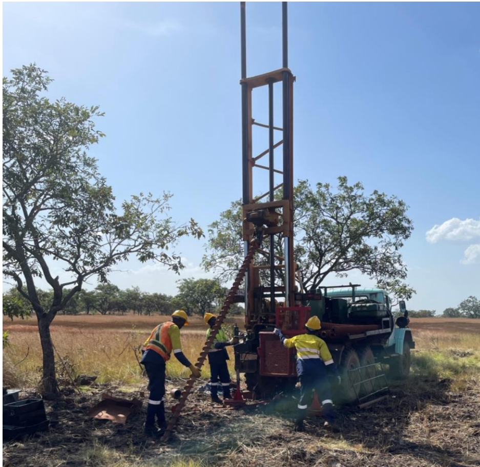
Figure 7. Auger drilling at Boussoura South
