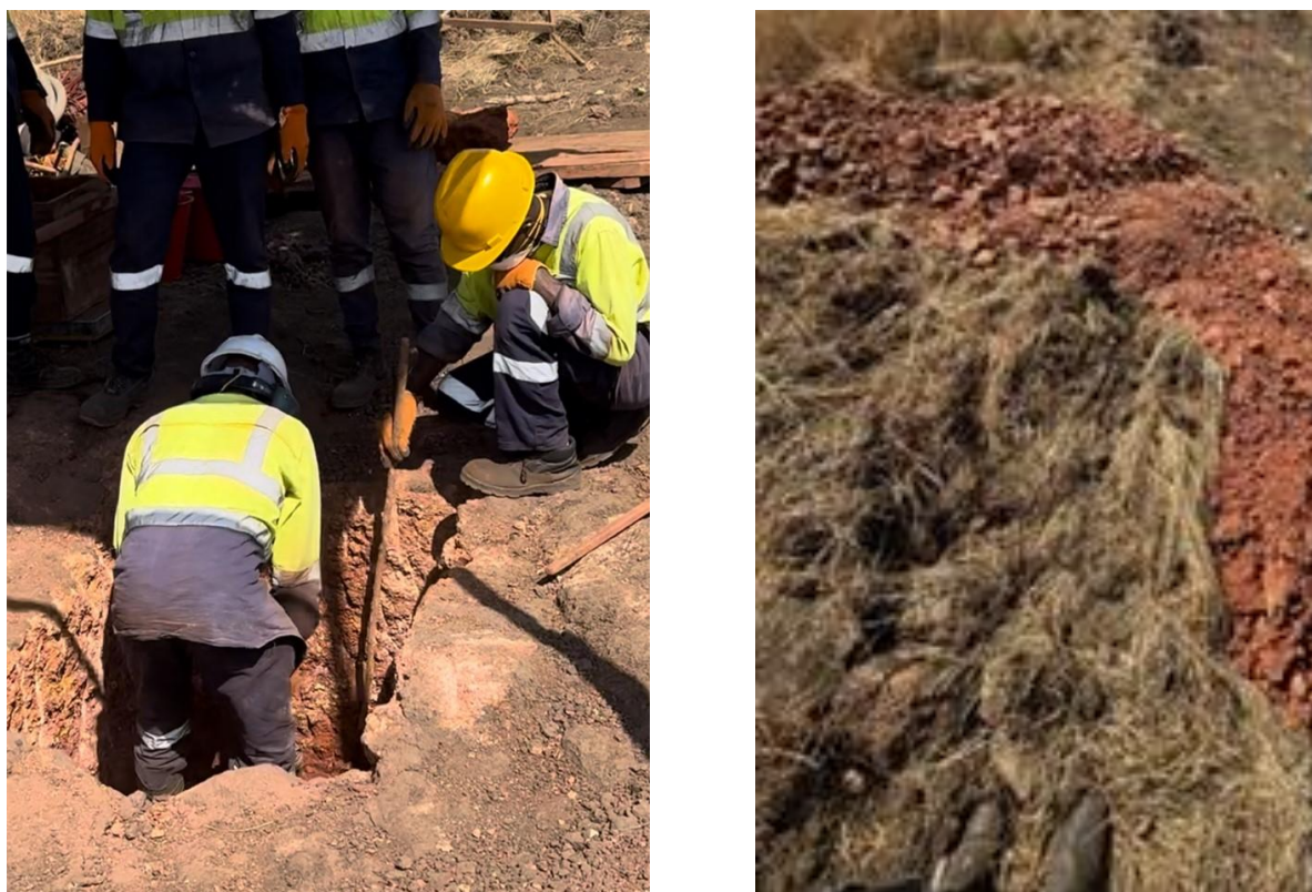
Figure 3. Shallow pits excavated left as part of collecting bulk samples displayed on right for ore characterisation test work.
