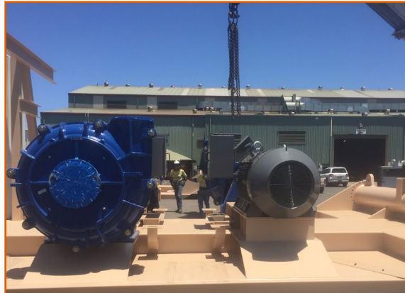
DMU Pump Skid Fabrication
