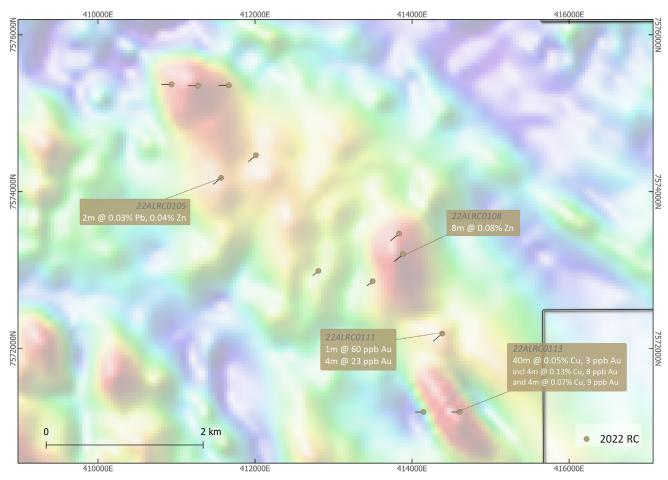
Figure 6. Flame Pea South Target showing RC holes on RTP aeromagnetic image
