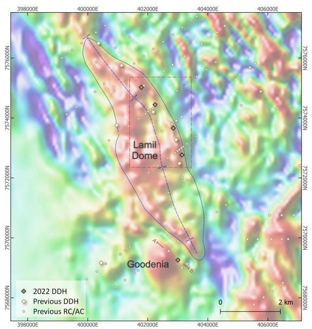
Figure 3. Location of Lamil Dome and Goodenia prospects on RTP aeromagnetic image
