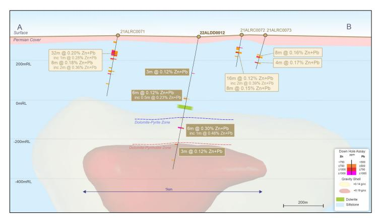
Figure 2. Oblique section of the Goodenia Prospect showing drill holes on geology with gravity shells defining density anomalism.
