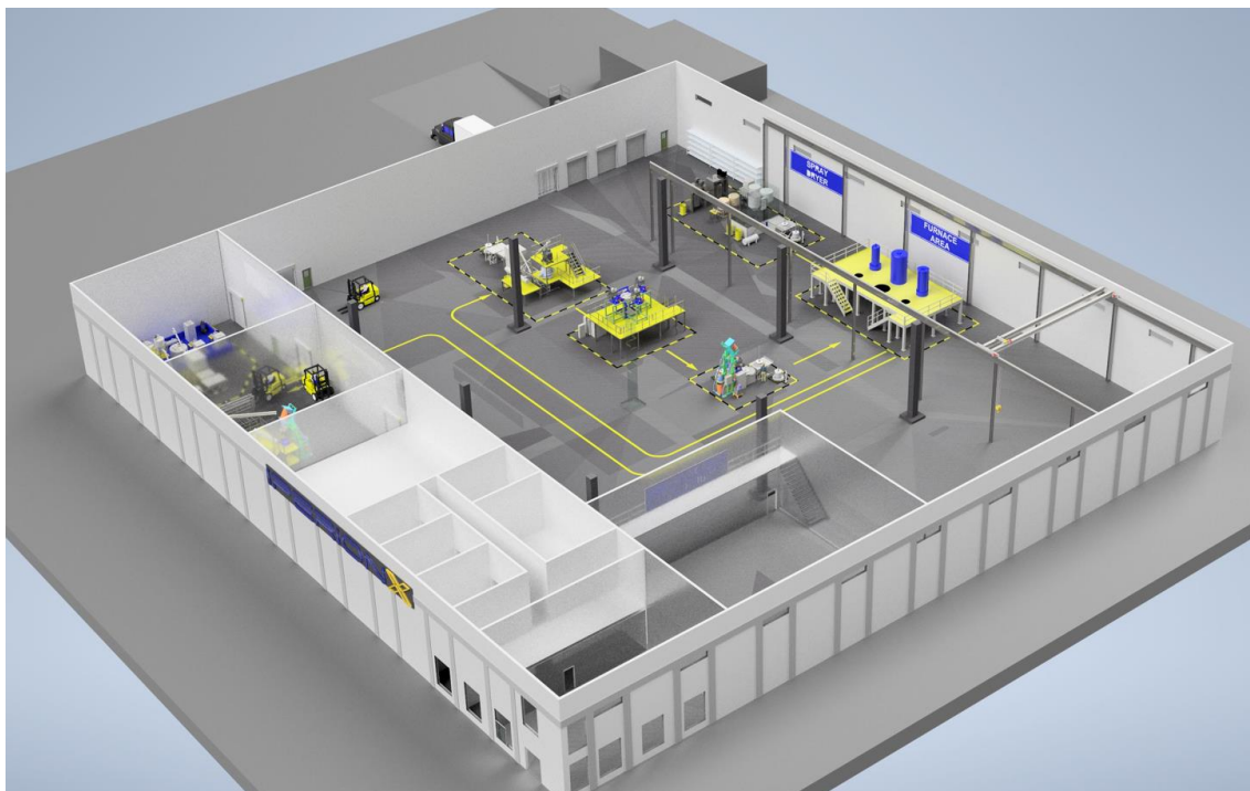
Figure 5: Isometric view of TDF 3D model, showing the spray drying and furnace areas with generic equipment for confidentiality reasons
