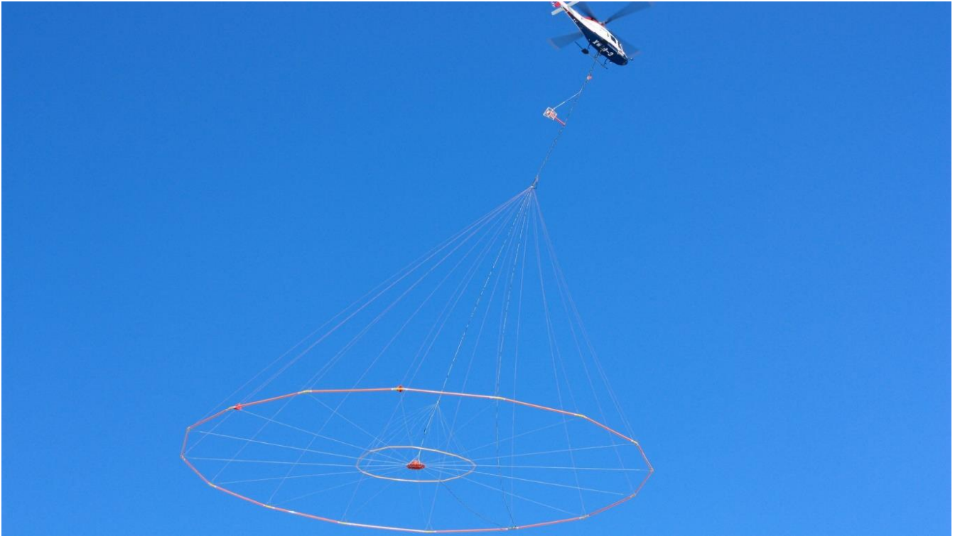
Figure 3: Helicopter Borne VTEM™ array
