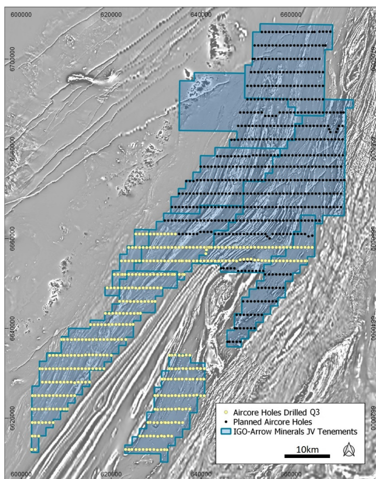
Figure 16: Aircore drill collars on greyscale aeromagnetic RTP 1VD image
