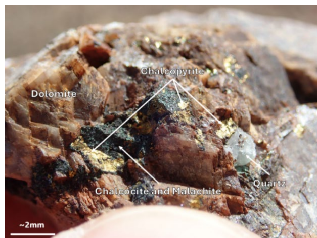
Figure 1. Quartz/Dolomite Vein with chalcopyrite, chalcocite and malachite. Worrumba 21 Mine Workings.
