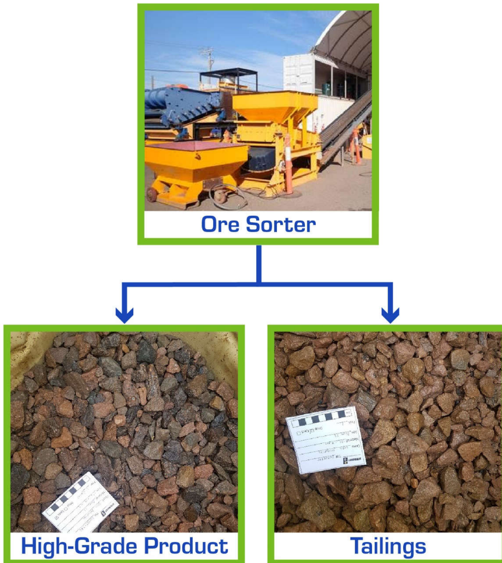
Image 2: Drum 26 finer feed being processed through the ore sorter before being separated into product and tailings
