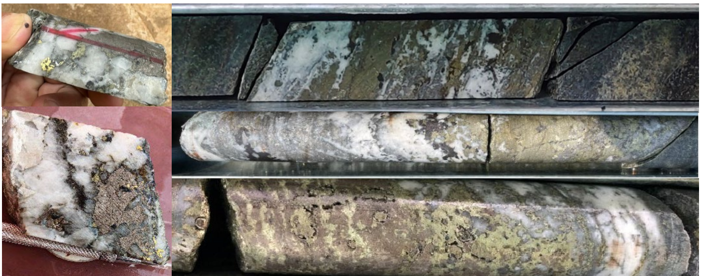
Figure 5 | Mineralised veins in Memot diamond core. Quartz veining with Pyrite, Arsenopyrite, Pyrrhotite, Chalcopyrite and Sphalerite sulphides. In order from Left hand Side photos: DD24MMT243 - 1m @ 2,090.00g/t Au from 130m. Right Hand Side Top to Bottom DD21MMT001 - 1m @ 8.91g/t Au, 2.16% Cu from 48m, DD22MMT013 - 0.4m @ 17.70g/t Au, 230g/t Ag, 2.78% Cu, 0.56% Pb and 1.74% Zn from 190m and DD21MMT006 - 1m @ 25.4g/t Au, 73g/t Ag, 1.81% Cu, 0.1% Zn
