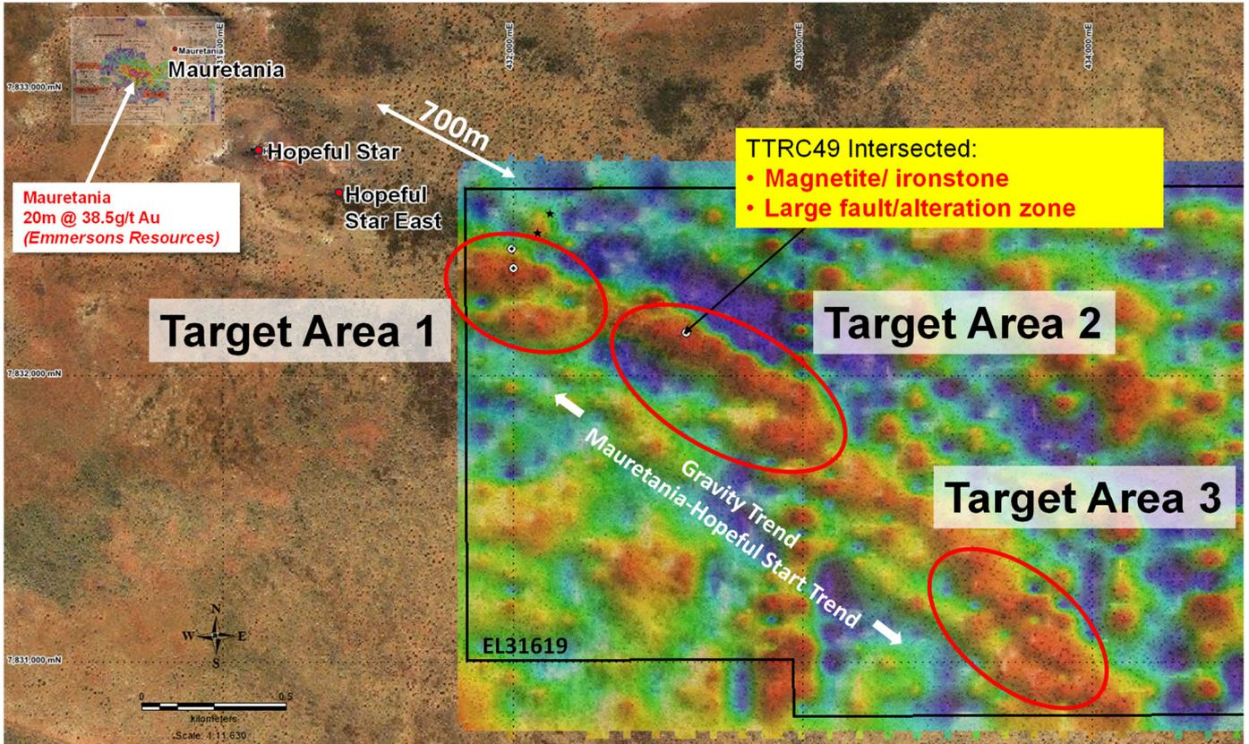
Figure 3: Mauretania/Hopeful Star trend into KRR's EL31619 at Langrenus, 3 main target areas with 3D inserts showing DDIP anomalies and gravity anomalies, translucent geophysical image is 1vd gravity.
