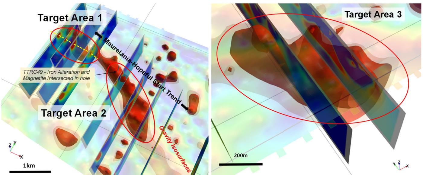
Figure 4: 3D view of DDIP sections at Langrenus. Red isosurfaces – gravity; coloured cross sections - DDIP chargeability; transparent surface - 1vd gravity image.
