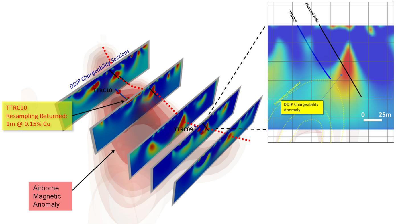
**Figure 2: DDIP lines across the Commitment airborne Magnetic anomaly where geochemically anomalous ironstones were intersected in previous RC holes. Proposed holes shown as black lines (final hole positions may change), previous drilling shown as blue lines.**
