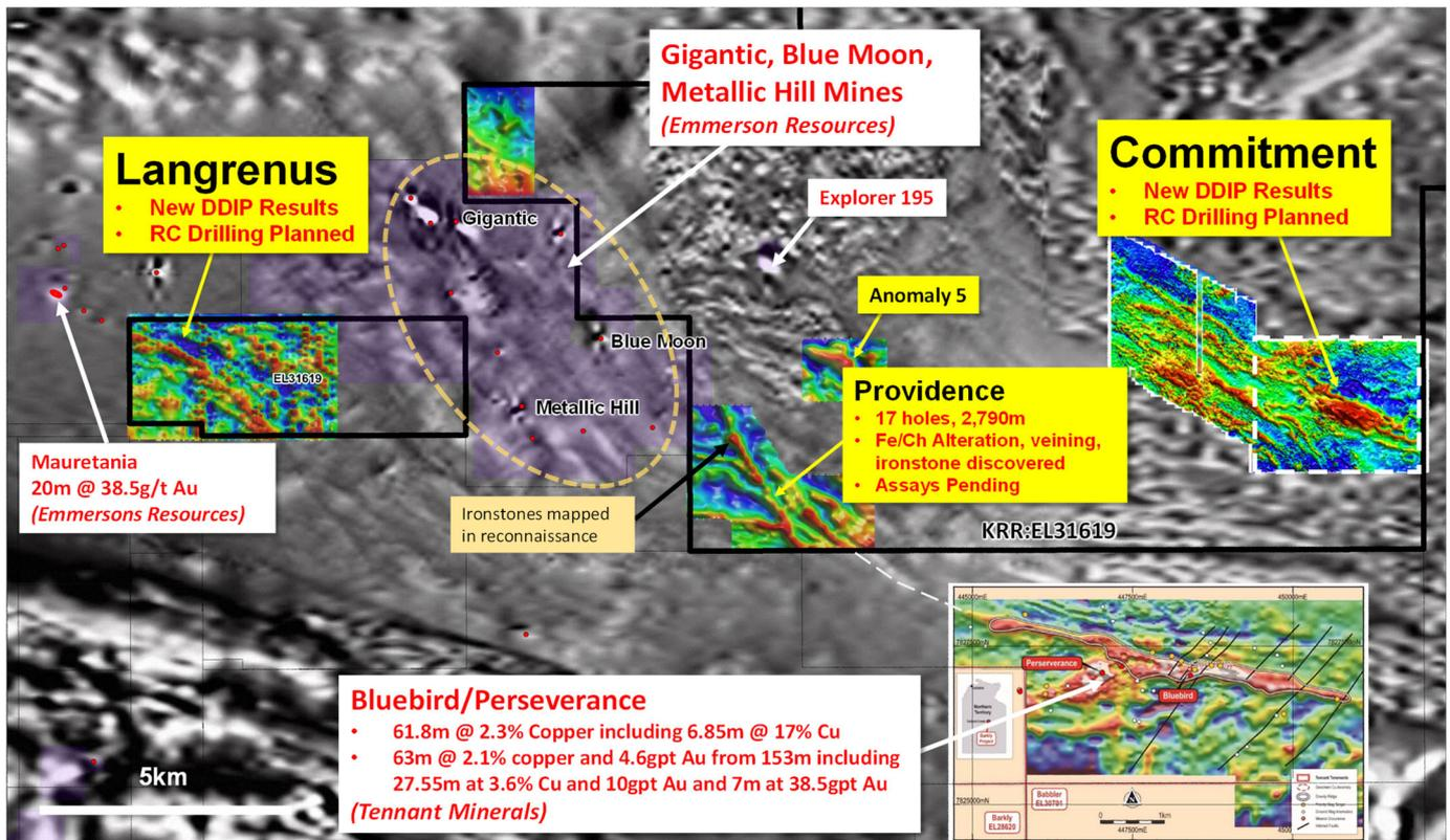
Figure 1: Location of Commitment and Langrenus in relation to Gigantic/Metallic Hill deposits, Mauretania and Tennant Minerals Bluebird-deposit. Magnetics (black and white) and gravity (coloured), insert is Tennant Minerals Gravity map.
