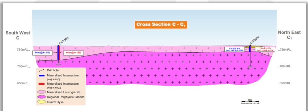
Figure 4: IP Conchas Cross Section C-C<sub>1</sub>
