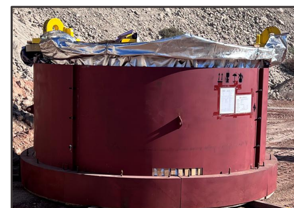
Ball mill trunnion on site
