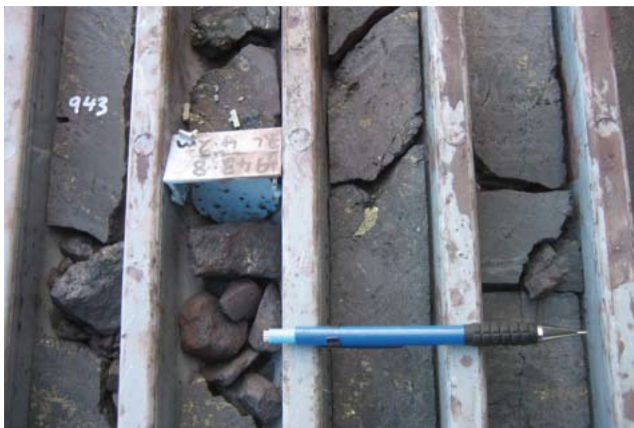
Drill core from hole MGD 55, 945m, showing massive hematite with minor copper sulphides
