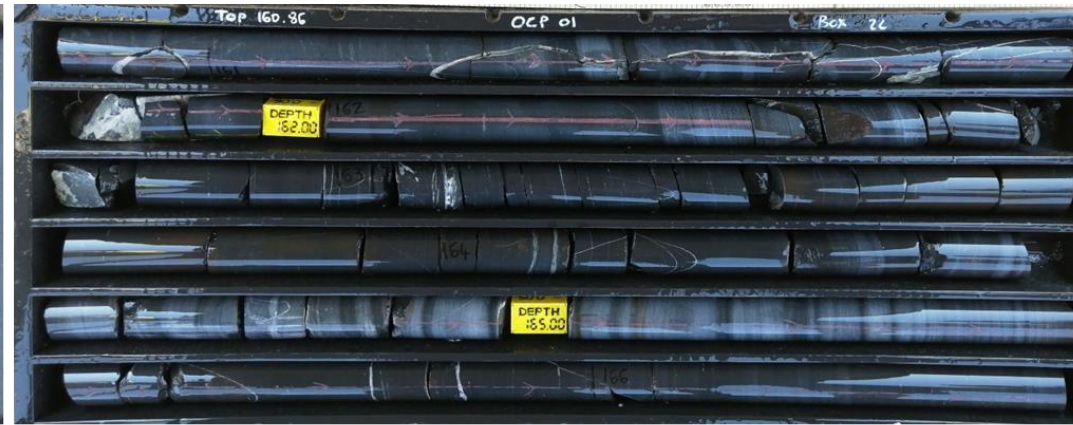
Conductive carbonaceous siltstone with light grey strongly calcareous zones from OCP01
