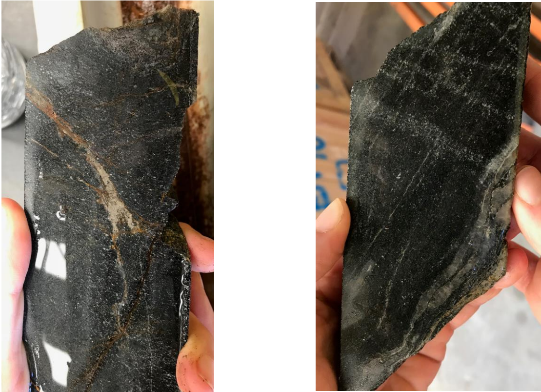
Figure 7 - Multiple generations of quartz and sulphide veining within mafic amphibolite host from BARDD002: 73.6m (73-74m grading 1.7 g/t Au) 56.0m (56-57m grading 2.9 g/t Au)
