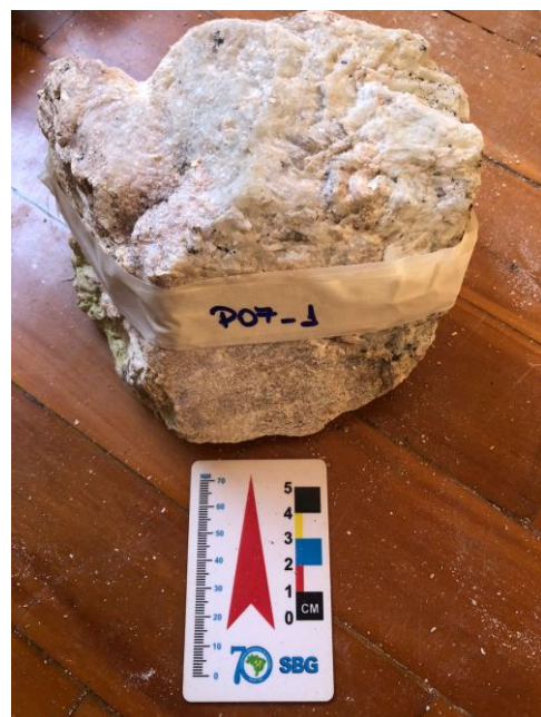
Photo 3: N Green fine-grained lepidolite + amblygonite sample (P07_1) from Mina Bom Jesus de Baixo, 2.66% Li 2 O
