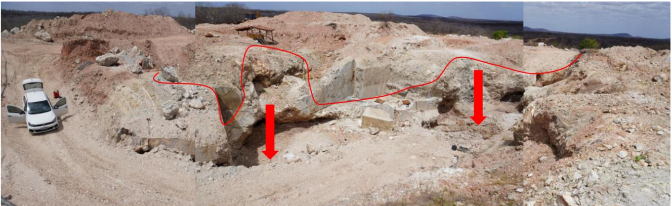
Photo 6: Mina Bom Jesus de Baixo quarry looking north (red line = pegmatite/country-rock contact; red arrows indicate dip direction of pegmatite) (refer footnote 2).
