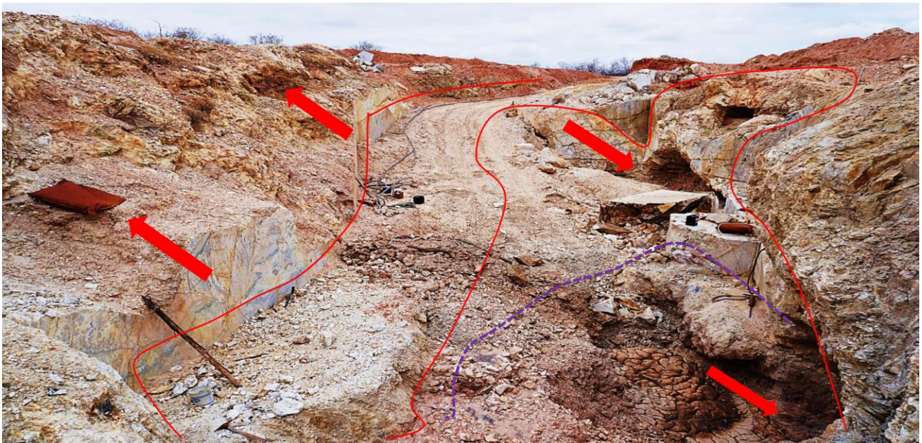
Photo 7: Mina Bom Jesus de Baixo quarry looking west. Note shallow dip to north and possible fold to south (red line = pegmatite/country-rock contact; red arrows indicate dip direction of pegmatite; purple dashed-line contact area of massive lepidolite) (refer footnote 2).
