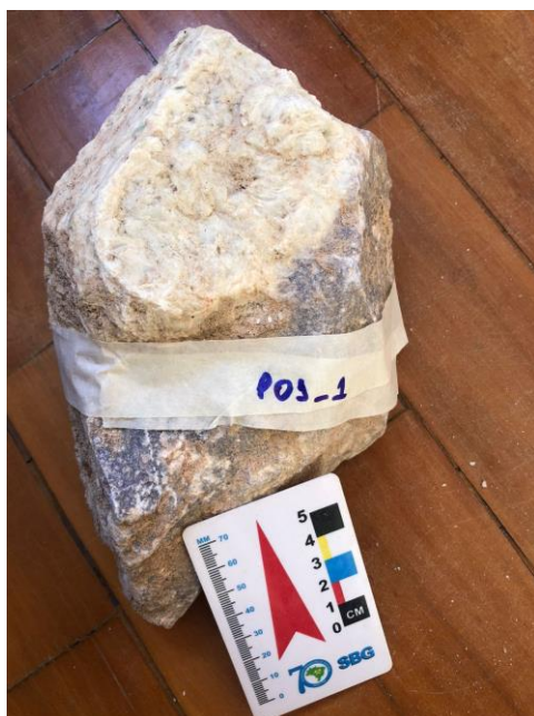
Photo 2: N Green fine-grained lepidolite + amblygonite sample (P01_1) from Mina Bom Jesus de Baixo, 2.64% Li 2 O (taken from same location as P01_2 shown on Figure 3)
