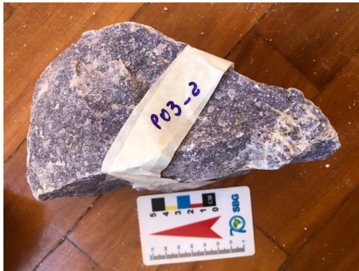
Photo 4: N Green fine-grained lepidolite sample (P03_2) from Mina Bom Jesus de Baixo, 4.25% \text{Li}_2\text{O}
