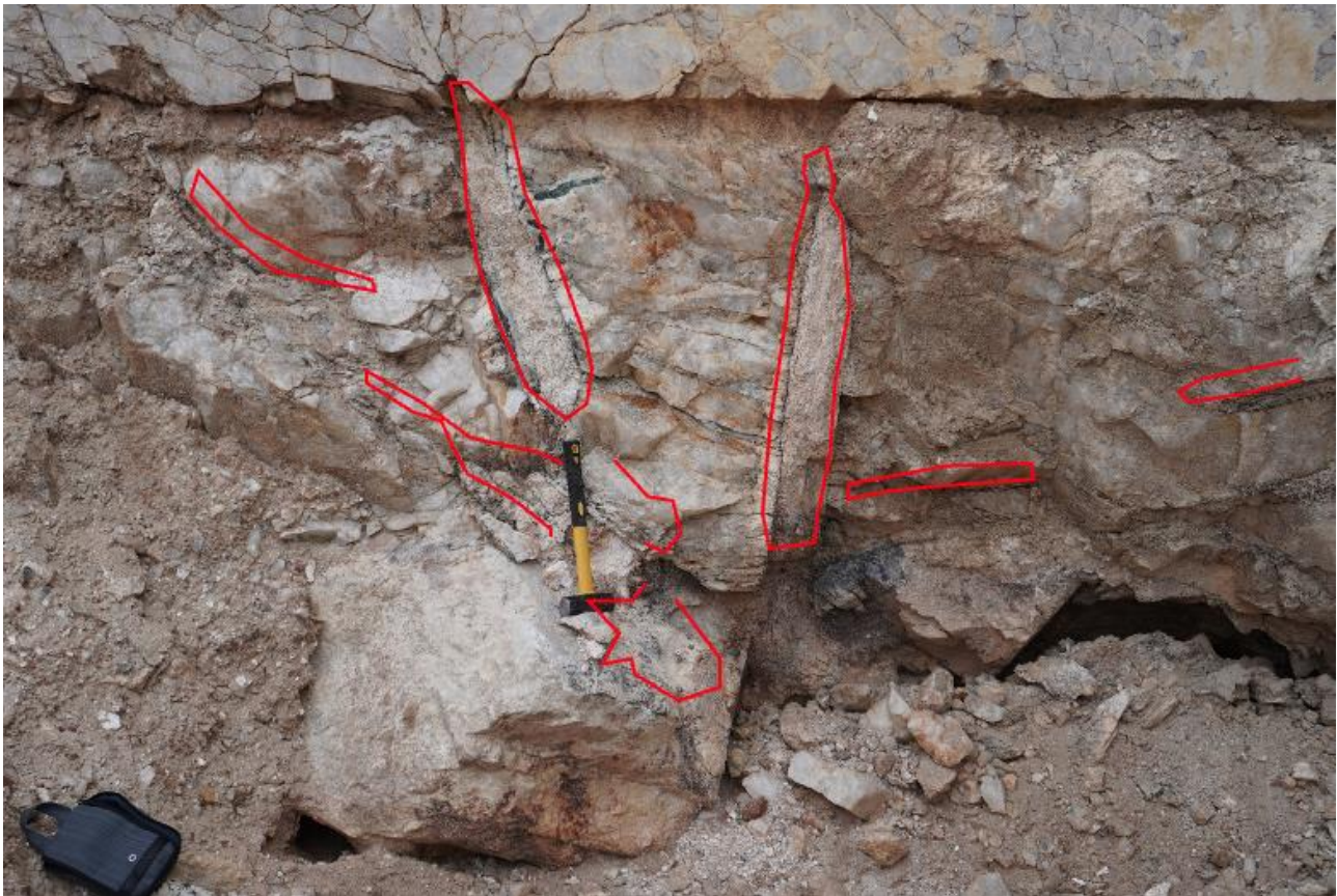
Photo 1: quarry face at Mina Bom Jesus de Baixo on permit 800306/2020 showing possible large spodumene crystals (red polygons) weathered to clays (sampled by Oceana, refer footnote 2).
