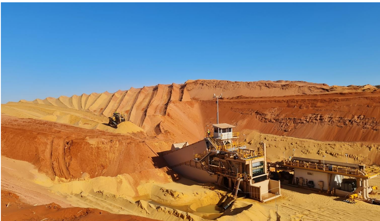
Figure 2 Coburn Project – Dozer Push Mining of Free-flowing Sand
