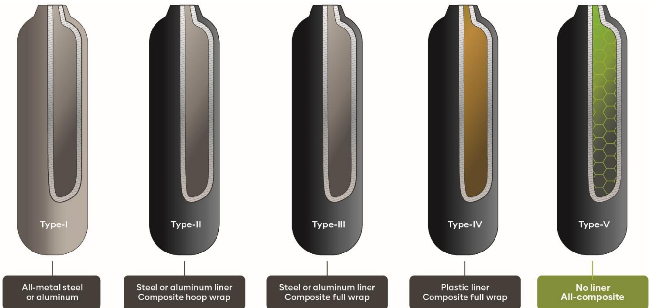
Figure 1: Five common pressure vessel types including Type-V tank.
