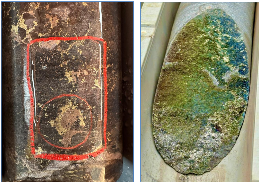
Figure 6. (Left) Net-textured chalcopyrite–pentlandite–pyrrhotite mineralisation in hole SWDD006 (226.55–226.85 m) showing interconnected sulfide networks within a magnetite-bearing mafic host, typical of magmatic segregation and coalescence of immiscible sulfide melt. (Right) Bornite–chalcopyrite sulfide band developed along a fracture plane in SWDD002 (86.7–89.42 m). Assays pending (refer ASX announcement dated 29 October 2025 for further details).
