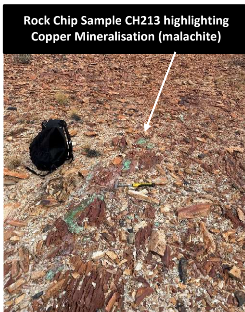
Figure 16 - Malachite eastern edge of 8-10m copper zone, strike 160° dip -30° west
