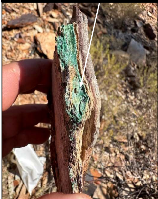
Figure 11 – Numerous stringers of malachite over 3m wide, -65° dip bearing 165°
