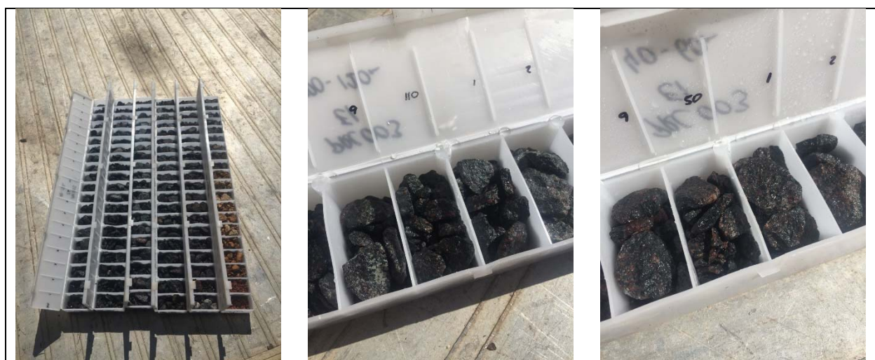
Figure 2: RC chip trays from PRC003 showing mafic rock samples
