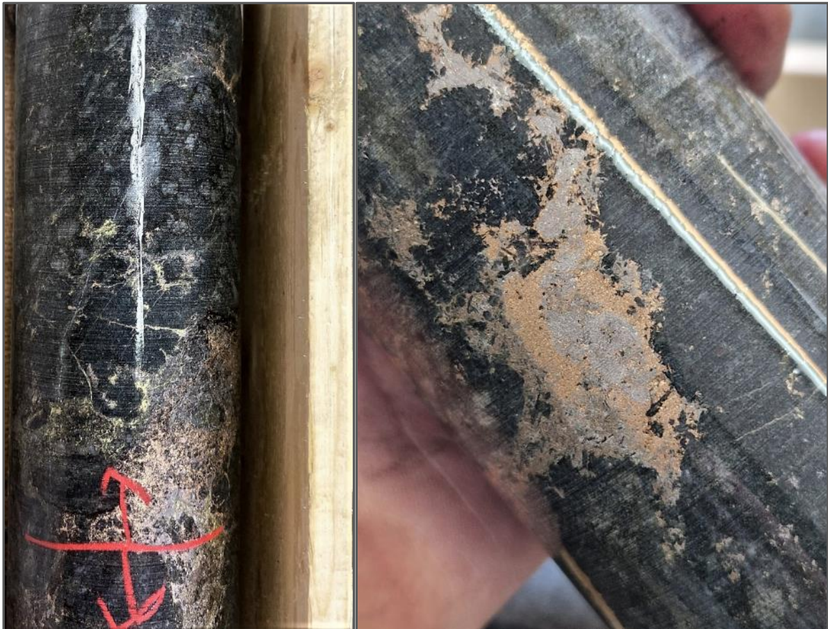
Figure 1: Lainejaur Project – Drillhole LAI23001, massive sulphides showing nickel-copper sulphides (pyrrhotite, pentlandite and chalcopyrite)
