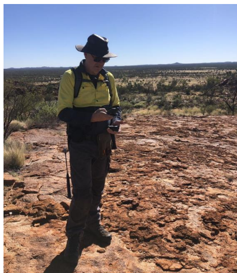
Figure 6: Graeme Fraser conducting field work within Oceana's EL32836, standing with a radioactive reading machine (Gamma-ray ( \gamma -ray) spectroscopy) at the granite tested by Callabonna Uranium Limited with shallow diamond drilling
