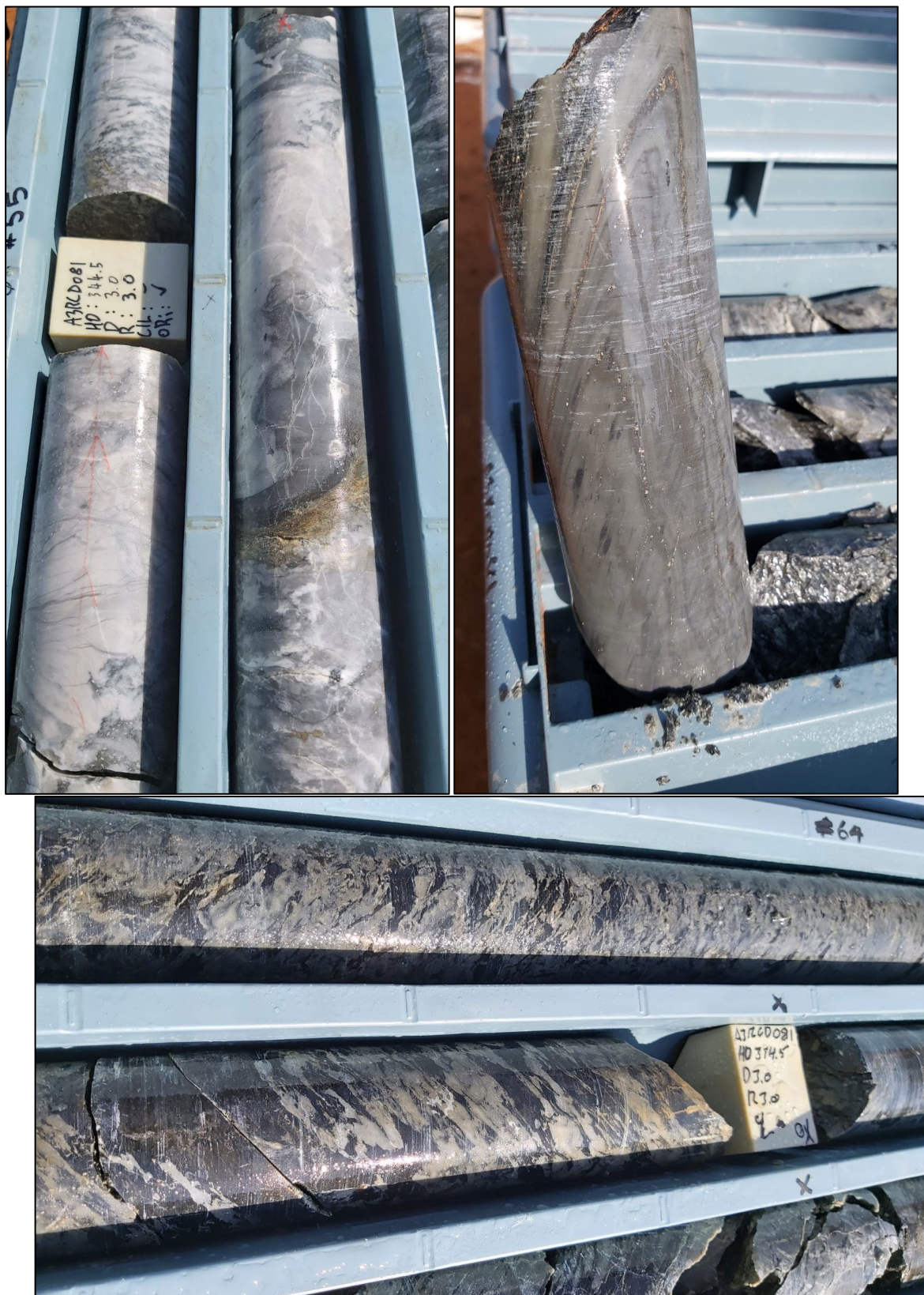
Figure 8: Various photographs of the important thinly bedded facies in A3RCD081 demonstrating the intensity of shearing, folding and silica alteration (top photos) and chlorite alteration (bottom).
