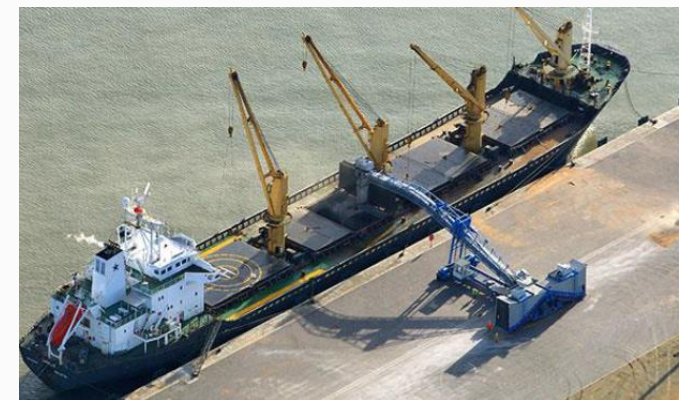
Image: Typical Mobile Dump Hopper and Shiploader
