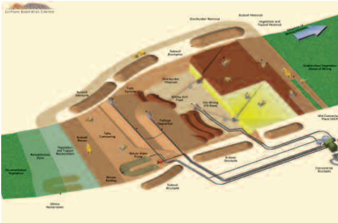
Figure 6. Amy Zone Mining Method
