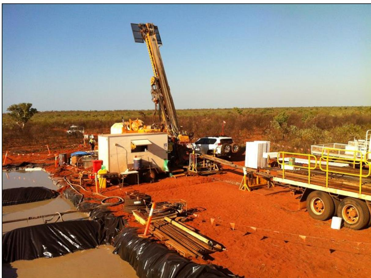
**Figure 11 – Drilling of diamond hole PAD001 at the Pardoo Nickel Project**
