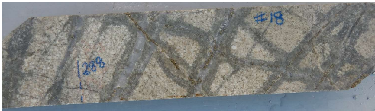
Fig 10. Example of typical “porphyry-style” multi directional quartz sulphide vein stockwork and sheeted veins with median hairline veins of pyrite, with quartz -sericite alteration selvages cutting a clast of sericite altered diorite .CAE Hole # 18 ,288m : Interval 288m-289m 1m @ 0.37 g/t Au, 0.03% Cu, 1.4 g/t Ag, 92 ppm Mo.
