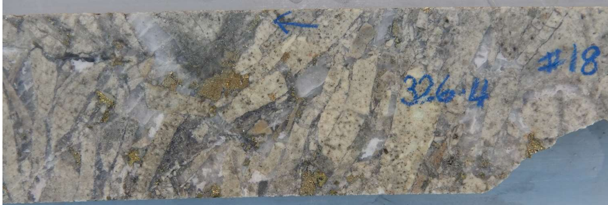
Fig 12. Photo HQ Half core, Infill Hydrothermal breccia with alignment of slab like clasts of sericite altered, diorite, hornfels. Infill calcite, quartz, pyrite, minor chalcopyrite. Hole # 18, 326.4m : Interval 326m-327m : 1m @ 0.22% Cu 0.14 g/t Au, 6 g/t Ag, 4.97% S, 128 ppm Mo
