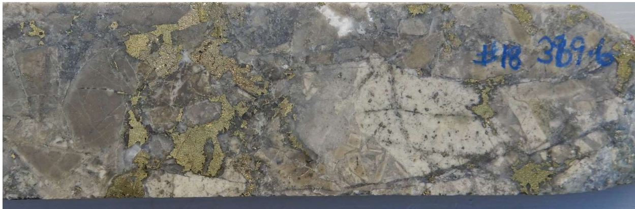
High copper section of sulphidic hydrothermal infill breccia CAE hole# 18 at 369.6m, Interval 369m-370m : 1m @ 2.99 % Cu ,0.33 g/t Au,33 g/t Ag , 6.77% S, translates to 1m @ 3.46% CuEq%.
