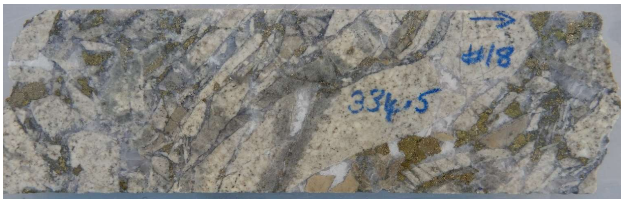
Fig 11. Photo HQ Half core, Infill Hydrothermal breccia with alignment of slab like clasts of sericite altered, diorite, hornfels . Infill calcite,quartz,pyrite ,chalcopyrite. Hole # 18 ,334.5m : Interval 334m-335m 1m @ 1.32% Cu 0.19 g/t Au, , 14.4 g/t Ag, 6.3% S, 270 ppm Mo.
