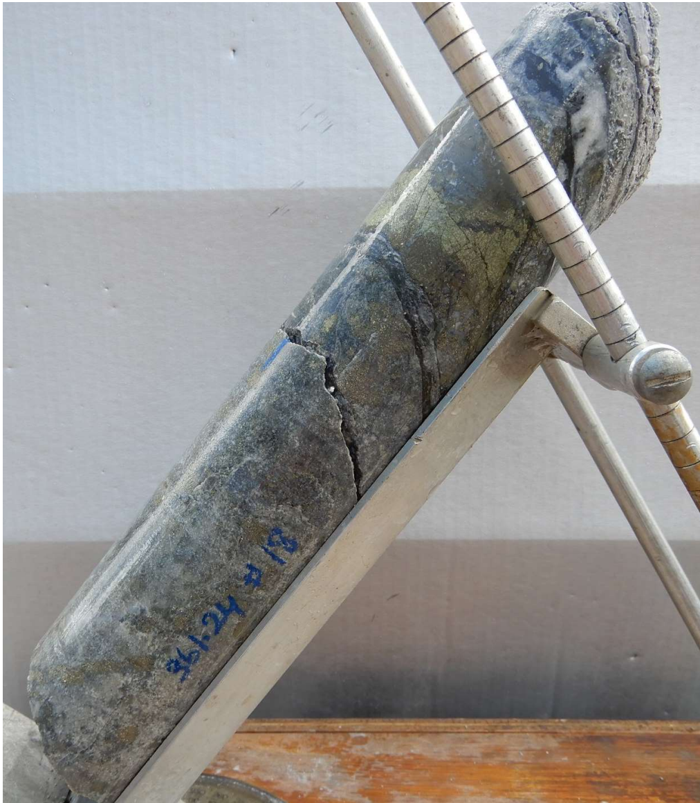
Fig 18. Photo HQ Full core, Hole #18 oriented in core oriented frame, hole drilling to south south west , view looking west north west. At 361m , hole inclined at -54 degrees toward 207 degrees mag. High grade gold section at top of core of semi-massive sulphide infill pyrite-chalcopyrite,galena,quartz,sericite vein/shear infill . Downhole contact with hydrothermal infill breccia ,strikes 280 degrees magnetic , dipping -78 degrees to north (dip direction 010 magnetic) . CAE hole# 18, 361.2m . Interval 361m-362m : 1m @ 10.8 g/t Au ,0.88% Cu,40 g/t Ag, 6.5% S..
