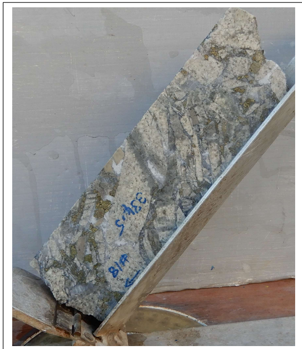
Fig 13 & 14. Photo HQ Half core, Hole #18 oriented in core oriented frame, hole drilling to south south west, view looking west north west. Fig 13. LHS Hole at 334.5m, Fig 14. RHS Hole at 326.4m, Hole inclined at -54 degrees toward 207 degrees mag. Alignment of slab like clasts oriented -75 dip towards 035 magnetic, strike 305 NW.
