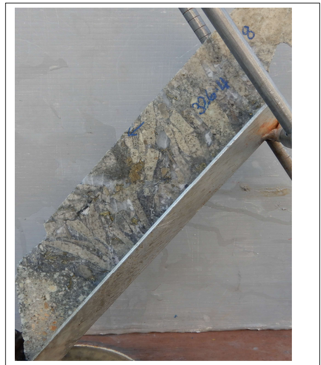
Fig 13 & 14. Photo HQ Half core, Hole #18 oriented in core oriented frame, hole drilling to south south west, view looking west north west. Fig 13. LHS Hole at 334.5m, Fig 14. RHS Hole at 326.4m, Hole inclined at -54 degrees toward 207 degrees mag. Alignment of slab like clasts oriented -75 dip towards 035 magnetic, strike 305 NW.
