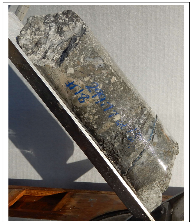
Fig 15. LHS. Photo HQ Full core, Hole #18 oriented in core oriented frame, hole drilling to south south west , view looking east south east. LHS Hole at 298.38m. Hole inclined at -54 degrees toward 207 degrees mag.. Contact of infill hydrothermal breccia uphole and light coloured argillised andesite downhole. Contact striking 285 magnetic bearing, dipping -50 degrees to 015 (NNE) dip direction..
