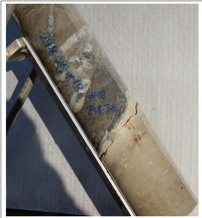
Fig 15. LHS. Photo HQ Full core, Hole #18 oriented in core oriented frame, hole drilling to south south west , view looking east south east. LHS Hole at 298.38m. Hole inclined at -54 degrees toward 207 degrees mag.. Contact of infill hydrothermal breccia uphole and light coloured argillised andesite downhole. Contact striking 285 magnetic bearing, dipping -50 degrees to 015 (NNE) dip direction..
