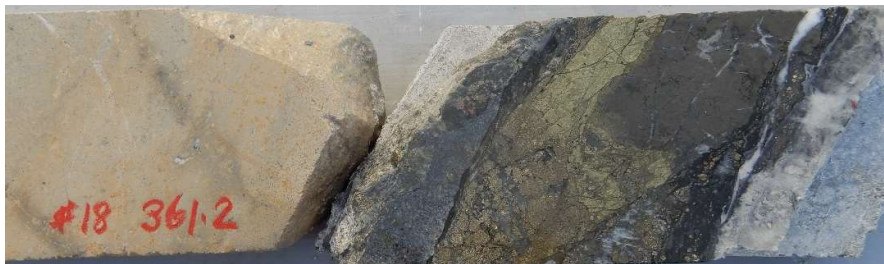
Fig 18. Photo HQ Full core, Hole #18 oriented in core oriented frame, hole drilling to south south west , view looking west north west. At 361m , hole inclined at -54 degrees toward 207 degrees mag. High grade gold section at top of core of semi-massive sulphide infill pyrite-chalcopyrite,galena,quartz,sericite vein/shear infill . Downhole contact with hydrothermal infill breccia ,strikes 280 degrees magnetic , dipping -78 degrees to north (dip direction 010 magnetic) . CAE hole# 18, 361.2m . Interval 361m-362m : 1m @ 10.8 g/t Au ,0.88% Cu,40 g/t Ag, 6.5% S..
