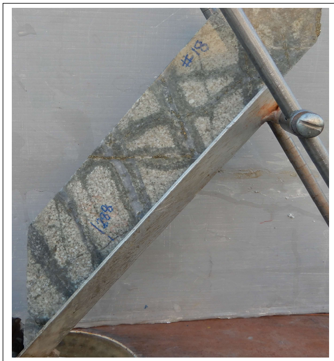
High copper section of sulphidic hydrothermal infill breccia CAE hole# 18 at 369.6m, Interval 369m-370m : 1m @ 2.99 % Cu ,0.33 g/t Au,33 g/t Ag , 6.77% S, translates to 1m @ 3.46% CuEq%.
