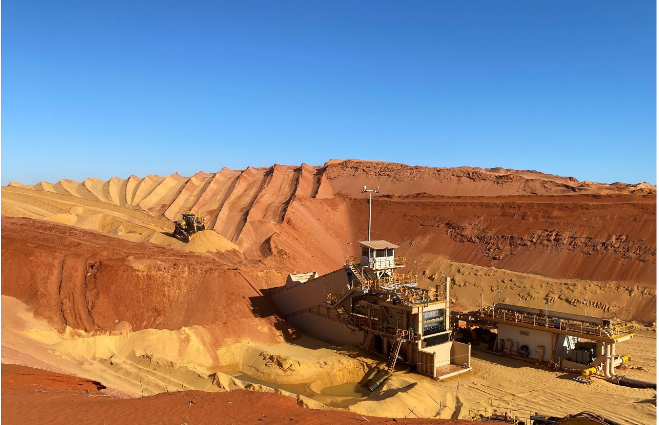
Figure 1 Coburn Project - D11 Dozer Pushing Ore into One-of-three In-pit Dozer Mining Units
