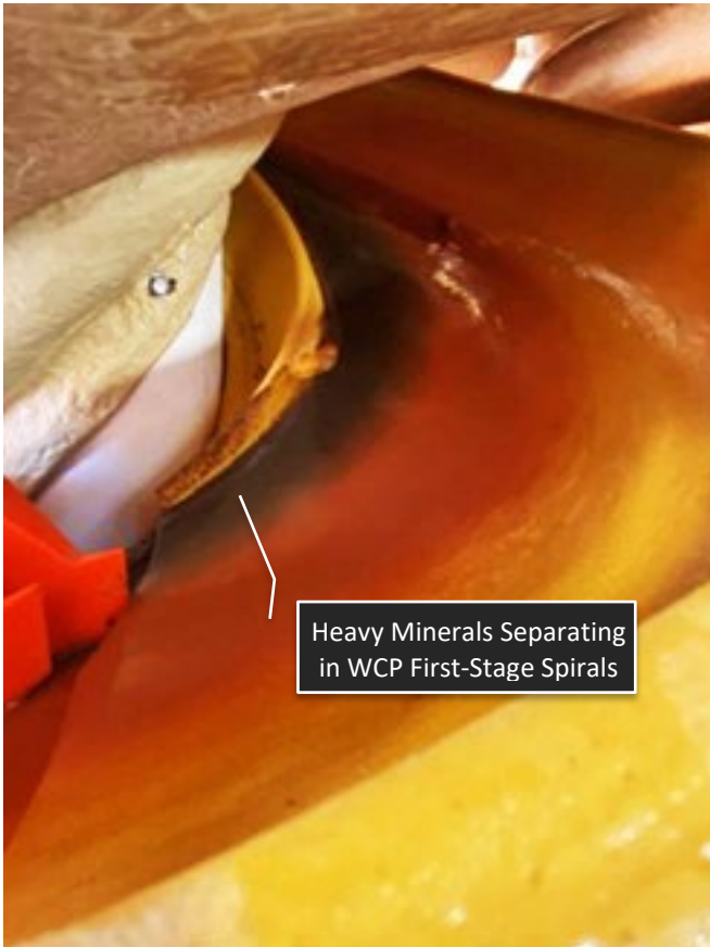
Figure 3 Gravity Separation of Valuable Heavy Mineral (dark colour) from the Non-valuable Sand in WCP First-stage Spiral Circuit
