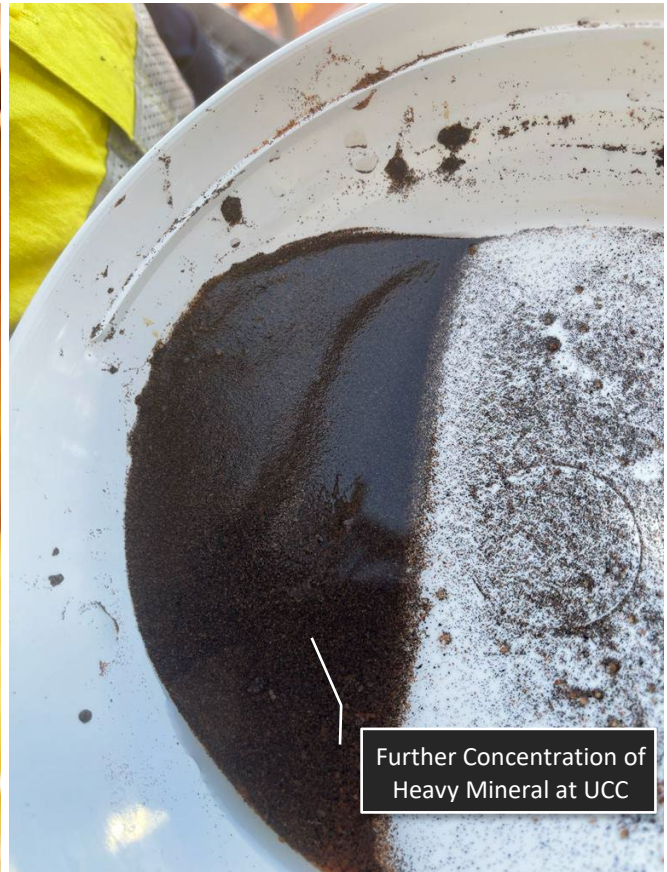
Figure 4 First Heavy Mineral Concentrate (HMC) at the WCP Upflow Classifier prior to Final Screening, Attritioning & Filtering
