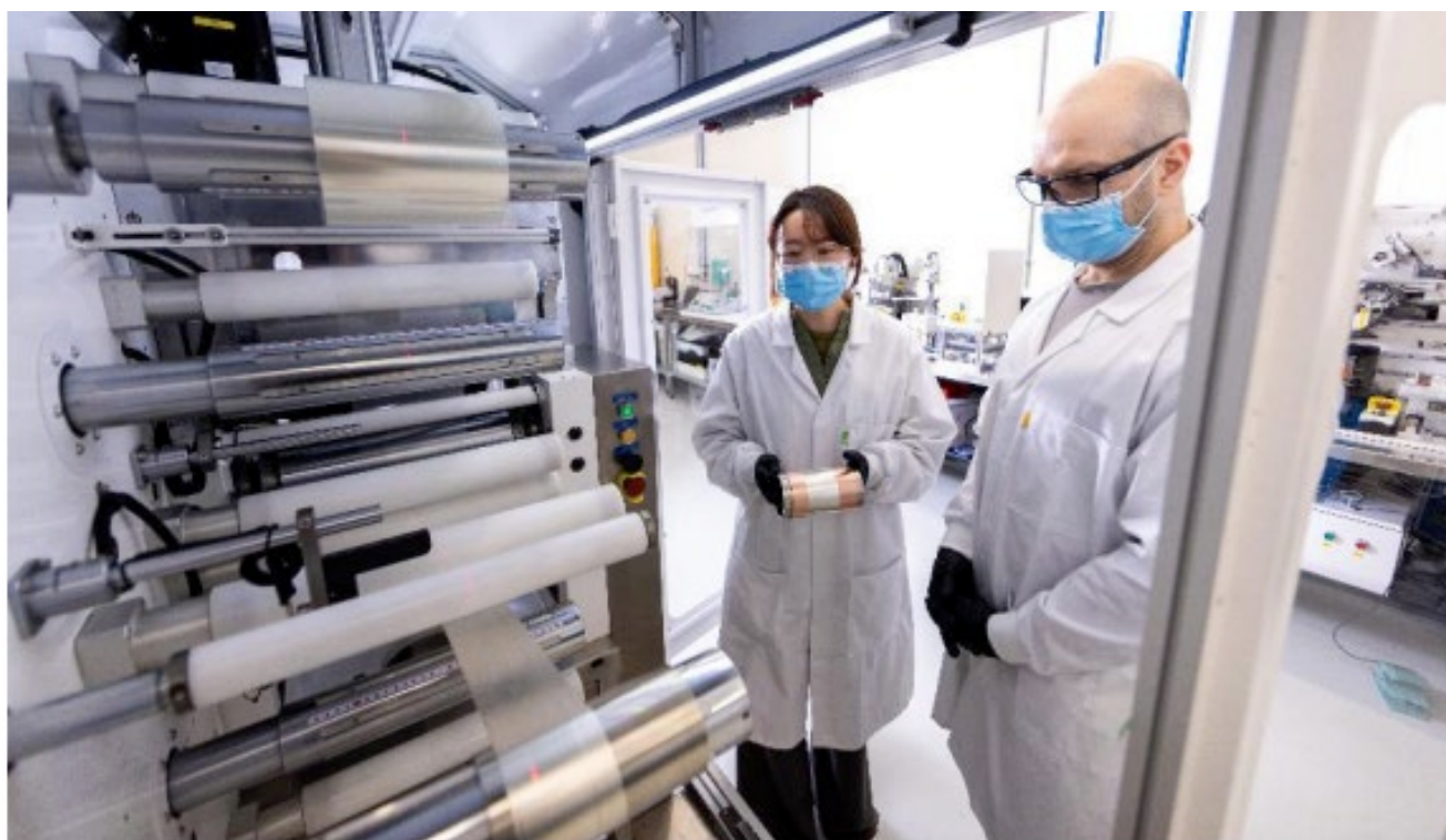
Li-S Energy staff monitoring the laminating process housed inside the Li-S Energy production dry room
